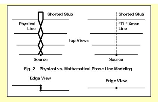
Essentially, we have two choices. We can attempt to model physically all aspects of the antenna array, as shown on the left in **Fig. 2**. Unfortunately, for NEC, this strategy quickly meets with some of the geometry limitations within the program. These limitations are functions of the calculation core and not of any particular implementation of NEC.
