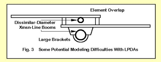
His phase line consisted of two tubes having different diameters. Ordinarily, the impedance of the line created by the two should be calculable from the diameter of the smaller tube, but the physical effects of the arrangement would be missing from the suggested modeling technique. In addition, he used muffler clamps to connect the lower element set to the larger boom. Most significant are
